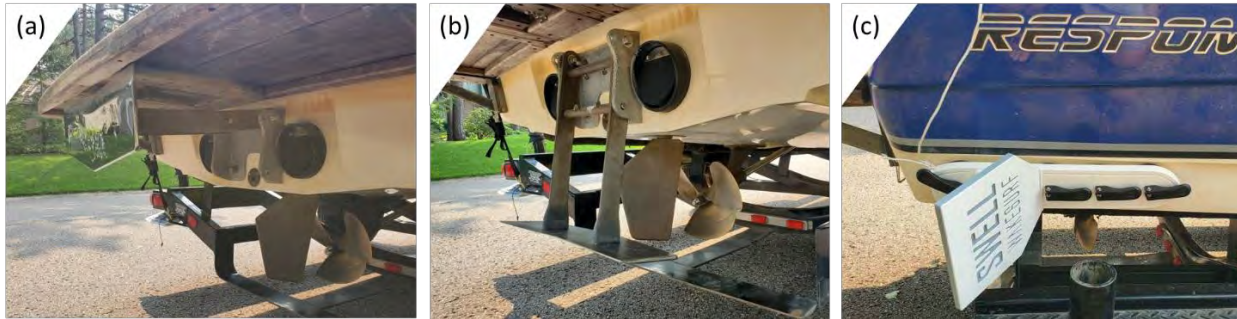
Figure 6. Malibu Response LX hydrofoil in the (a) stow position and (b) deployed down position. (c) Installed aftermarket wake shaper (Swell Wakesurf- Wakesurf Creator 2.0).
