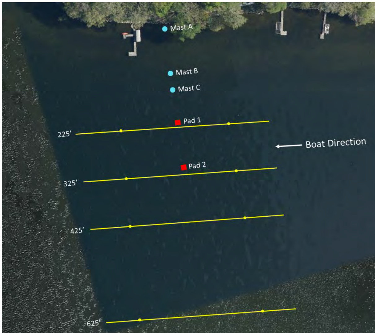
Figure 3. Layout of the study site. The three blue circles and two red squares indicate the locations of the masts and pads, respectively. The yellow lines show the distance of the boat track lines from the shoreline.
